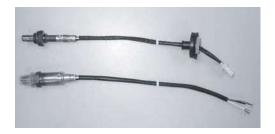
**Step 4:** Cut the wiring of OE Sensor 4" from end of connector as illustrated. Lay the Bosch Universal Oxygen Sensor beside the OE Sensor and cut the Bosch Universal Oxygen Sensor wiring to the length of the OE Sensor. Proceed to Step 6.
