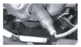
**Step 2:** If there are special clips or grommets attached to the OE Sensor, proceed to Step 3. Otherwise, if the length from the hex/flange face to end of OE Sensor connector housing is less than 29 1/2", proceed to Step 4, otherwise, proceed to Step 5.
