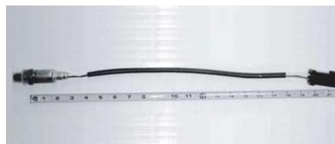
**Step 3:** Cut the OE Sensor harness so as to include special clips or grommets. Lay the Bosch Universal Oxygen Sensor beside the OE Sensor and cut the Bosch Universal Oxygen Sensor wiring to the length of the OE Sensor, but do not cut to less than 5" (hex/flange face to end of sensor wire). Proceed to Step 6.
