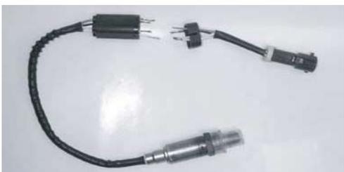
**Step 8:** Install a wire seal over each wire so that the unribbed end of the seal is facing the Connector Body and Cap. Check that the wires are aligned properly before proceeding.
