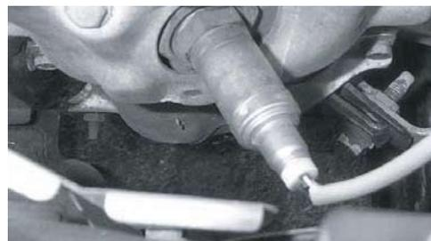
**Step 2:** If there are special clips or grommets attached to the OE Sensor, proceed to Step 3. Otherwise, if the length from the hex/flange face to end of OE Sensor connector housing is less than 29 1/2", proceed to Step 4, otherwise, proceed to Step 5.
