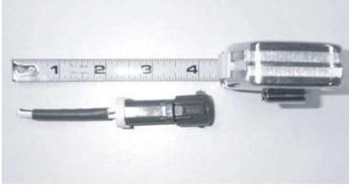
**Step 5:** Lay the OE Sensor beside the Bosch Universal Oxygen Sensor and cut the OE Sensor wires to the same length as the Bosch Universal Oxygen Sensor length. Cut the wire tie from the end of the Bosch Universal Oxygen Sensor wiring. Proceed to Step 6.
