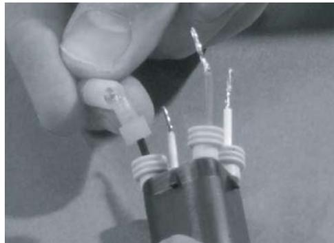
**Step 10:** Utilizing "Wire Color Reference Table", begin connecting the wires of the OE Sensor connector harness as described in Step 7. Be sure to avoid criss-crossing the wires. Grasp the wire on each side of the Posi-Lock connector and pull firmly to insure proper assembly.
